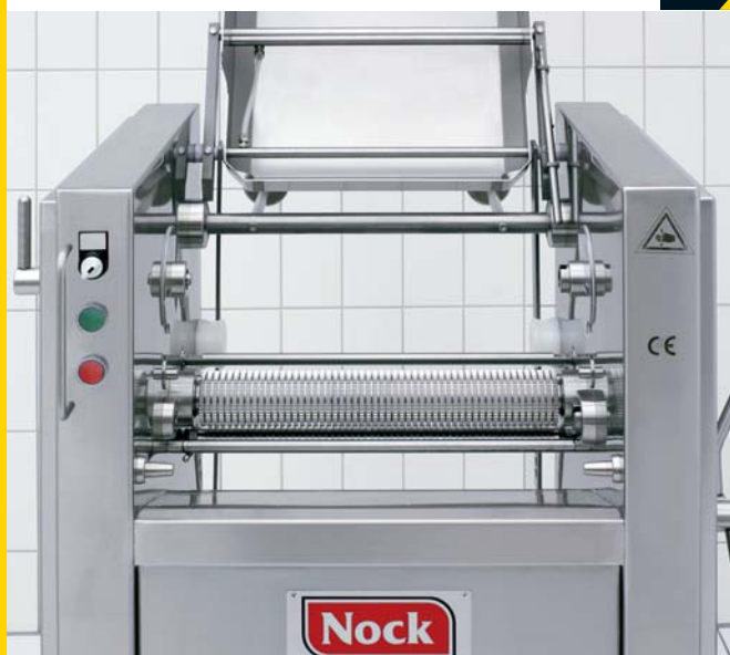
Quick and easy to clean: NOCK fish skinning machine after removing conveyor belts, pressure roller and blade holder
