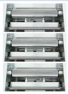
**NOCK Air Jet compressed air cleaning system:**Jet bar moved by an enclosed pneumatic cylinder
