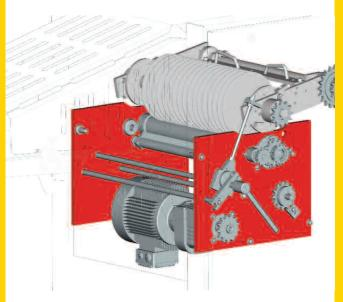
As every blade has to do less cuts, the blades last much longer than with other cutting machines. Depending on the product, ca. 500 - 1000 tons can be cut before the blades must be resharpened.
